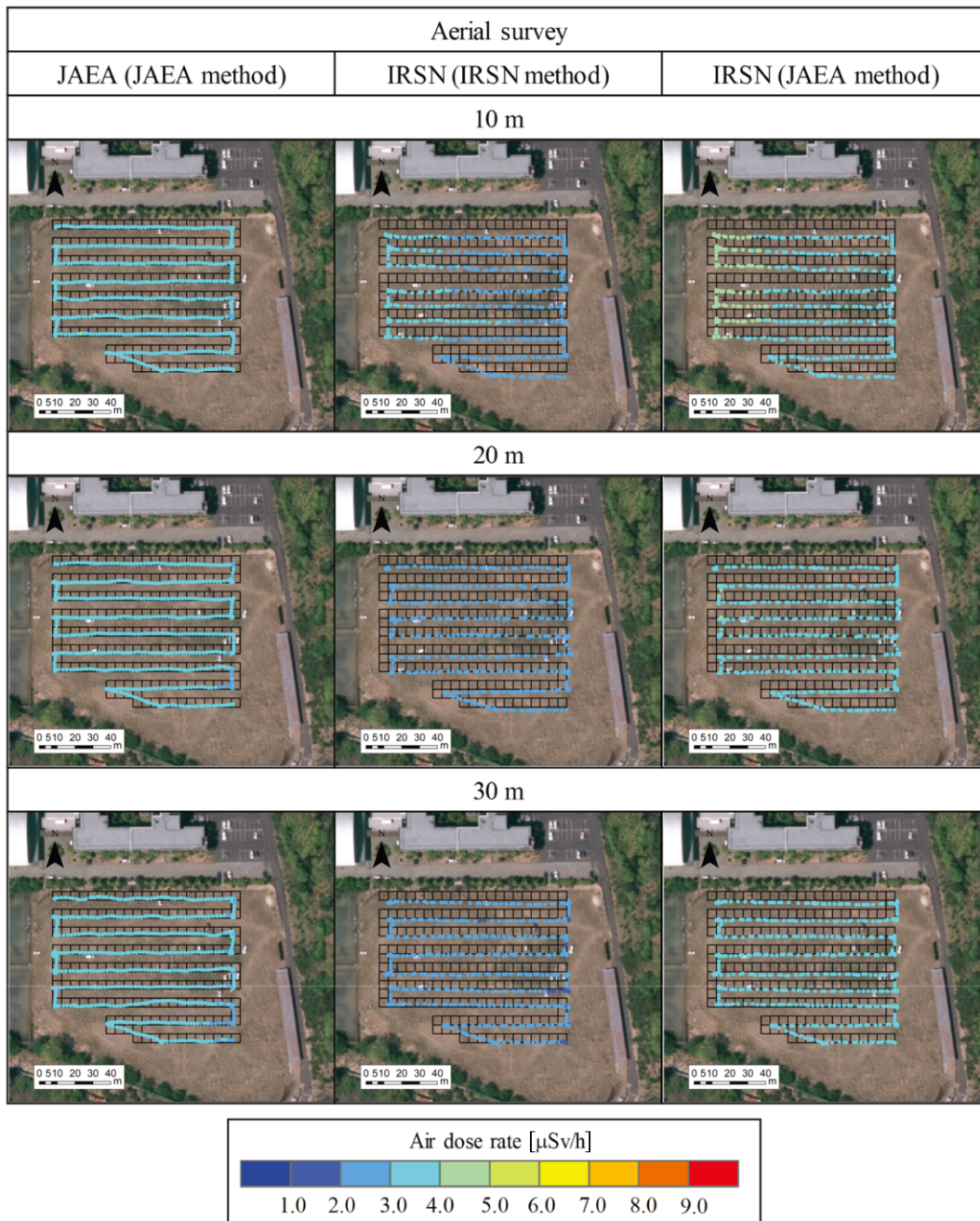
Fig. 10. Distribution of air dose rates at 1 m agl. obtained by airborne survey in site A. This map was created using ArcGIS 10.6.1.
