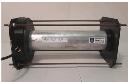
Fig. 1. The compact spectrometer. A 6 mm × 6 mm × 120 mm prism of EJ-276 scintillator is encased in an aluminium tube and coupled to a single SiPM housed in a 3D-printed casing.
